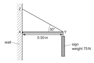
The frame consists of a horizontal rod XY and a rod YZ that is at an angle of 30° to the horizontal. Rod XY is attached to the wall by a hinge at X and has length 0.50 m. Assume that the weights of the rods are negligible.
