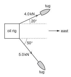
The tensions in the towing cables are 4.0 kN and 5.0 kN.
