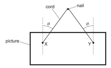
The tension in the cord is T. The angle between the cord and the vertical is  $\theta$  on both sides.
