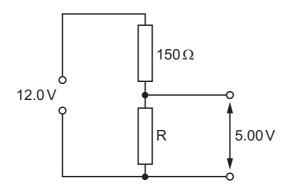
What is the resistance of resistor R in the potential divider circuit?
